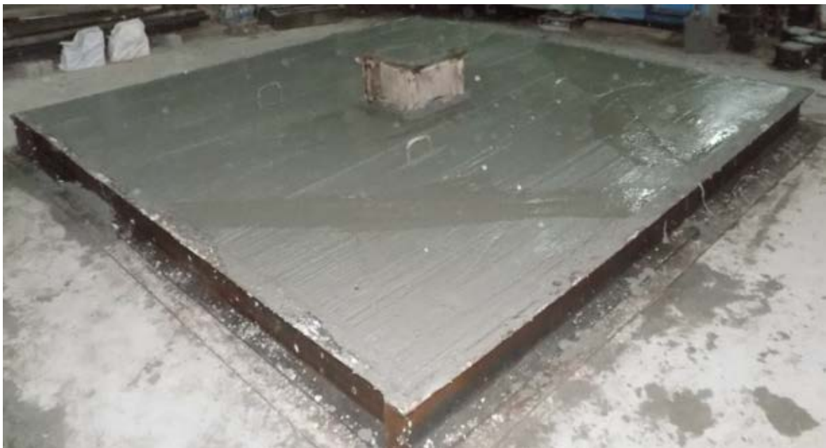
Figure 4.11 – Typical Punching Shear Test Specimen after Cast
