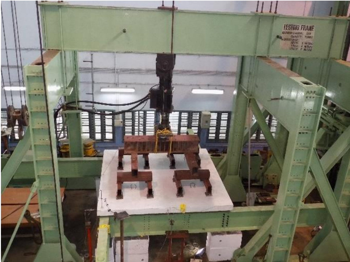
Figure 3.30 – Two-way Flexural Test Set-up: Phase I (Load up to 1000 kN)
