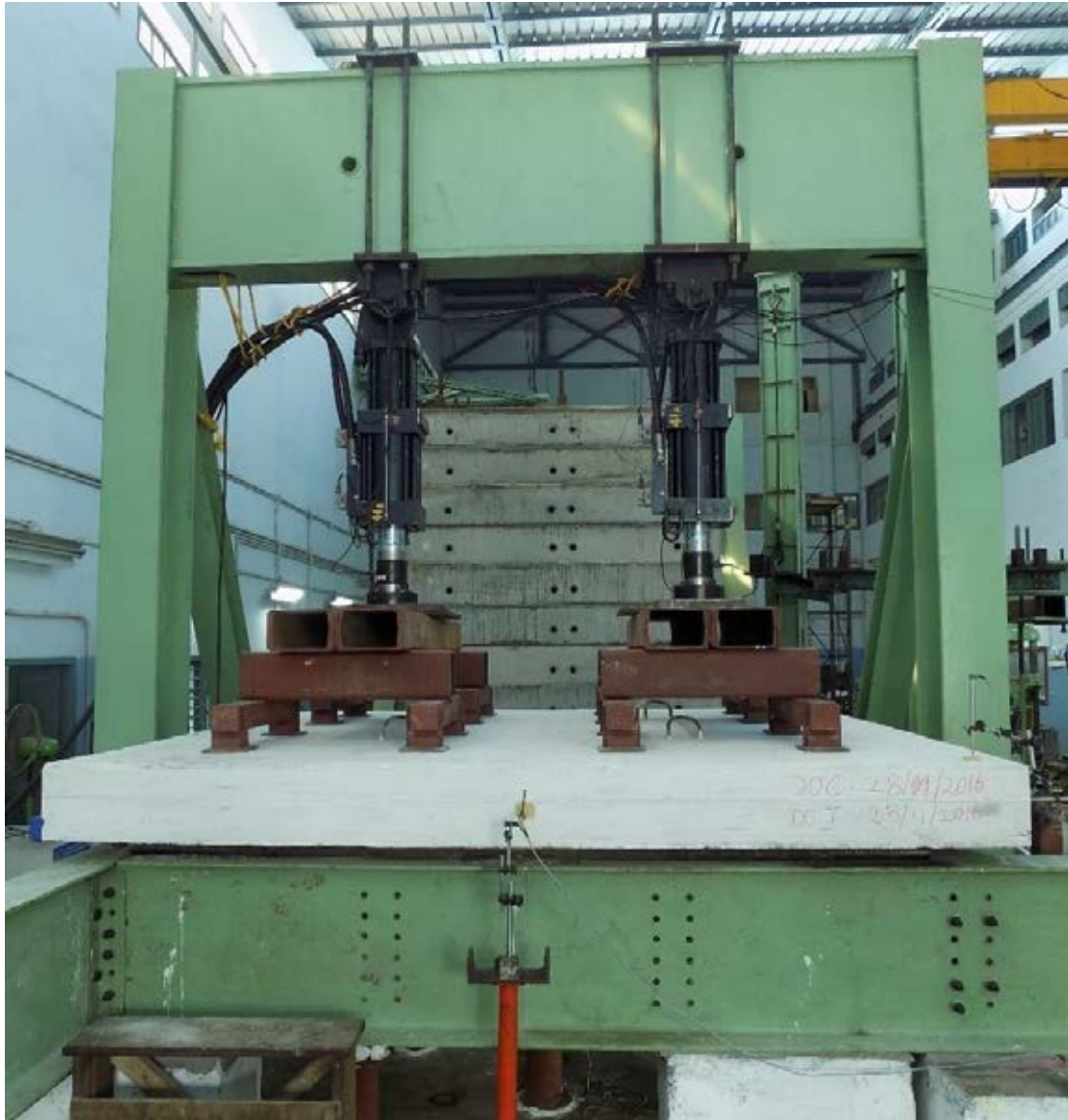
Figure 3.32 – Two-way Flexural Test Set-up: Phase II
