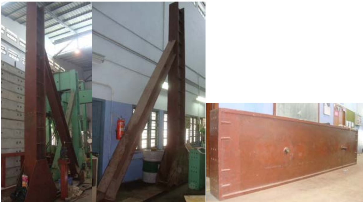
(a) Loading Frame Components – 'A' Frames and Box Girder
