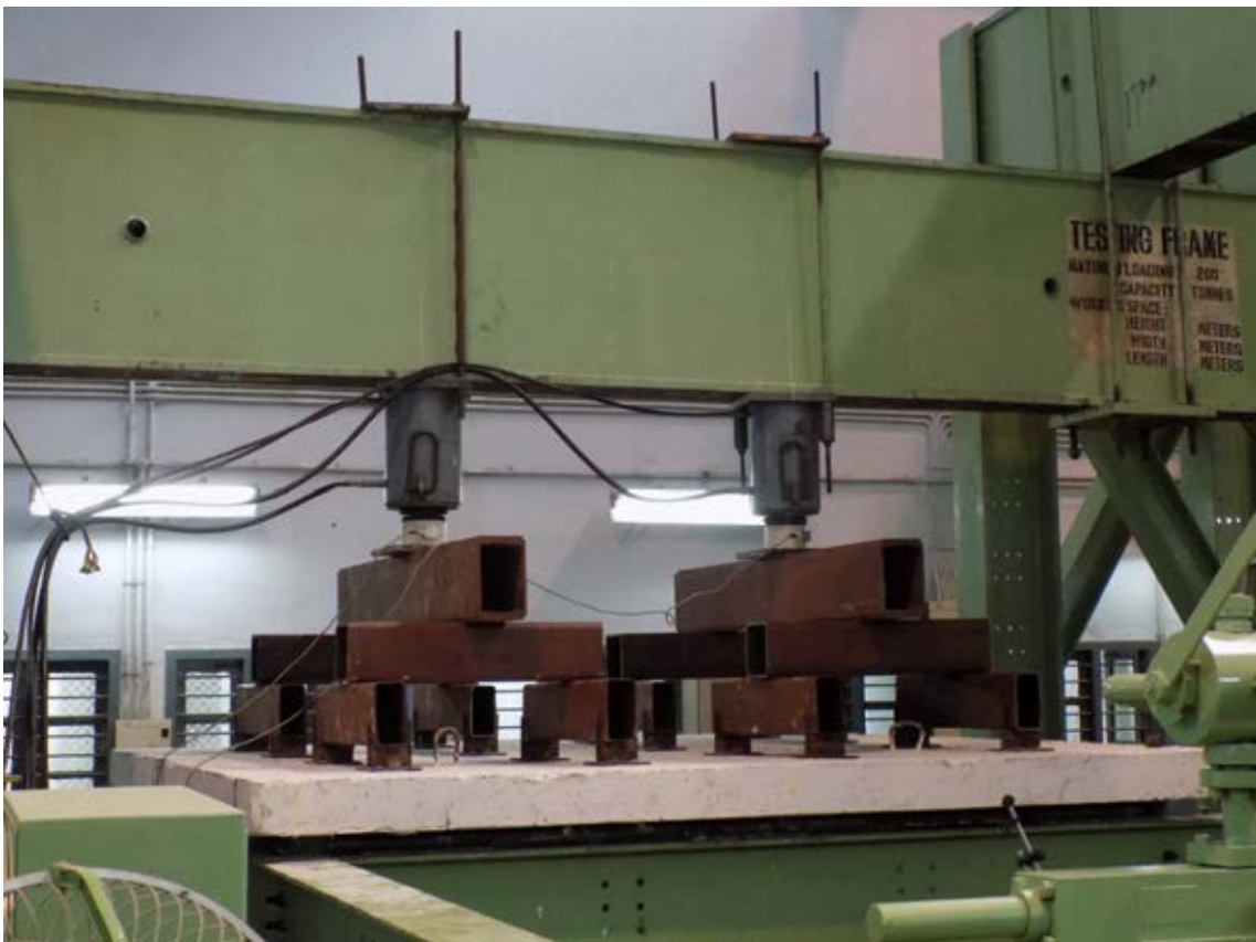
Figure 3.31 – Two-way Flexural Test Set-up: Phase I (Load up to Ultimate)
