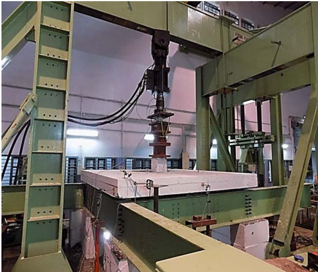
Figure 4.13 – Punching Shear Test Set-up: Phase I
